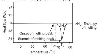
Fig. 2.1: Typical DSC Thermogram for Melting Point of Solid
