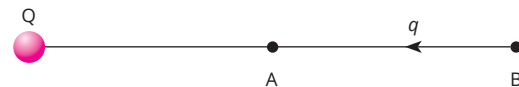
Fig. 1.7 Potential difference is the amount of work done in moving a unit charge q from point B to point A in an electric field created by the charge Q .
