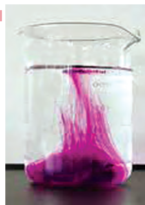
Figure 2. This picture shows the diffusion of potassium permanganate in water.
