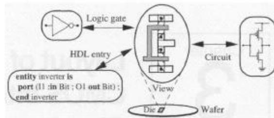
Figure 3.1. Equivalent descriptions of a digital integrated circuit.
