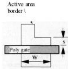
Figure 3.10. Gate spacing from an n<sup>+</sup> edge.
