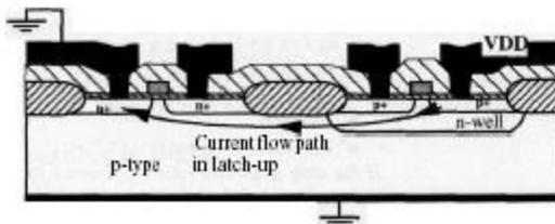
Figure 3.28. Origin of the latch-up problem in CMOS.
