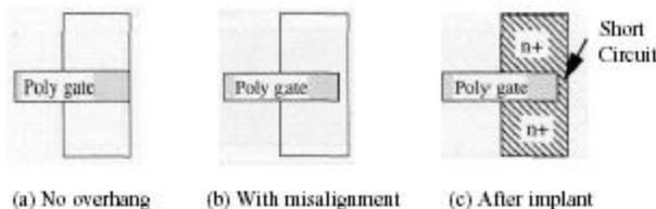
Figure 3.9. Effect of gate misalignment without overhang.
