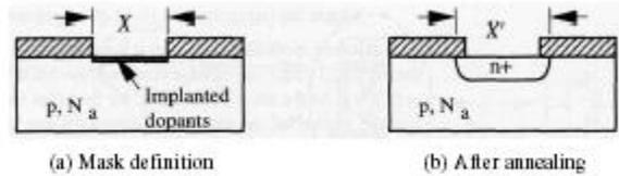
Figure 3.3. Patterning sequence for a doped  $n^+$  line.
