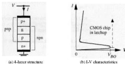
Figure 3.29. Four-layer (pnpn) device characteristics.
