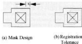
Figure 3.6. Contact spacing rule.
