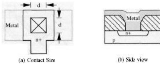
Figure 3.5. Geometry of a contact cut.
