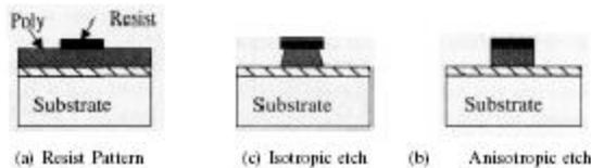
Figure 3.11. Polysilicon etch profiles.
