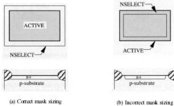
Figure 3.7. Formation of n<sup>+</sup> regions in an n-channel MOSFET
