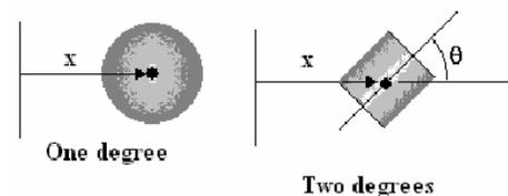
This needs only one dimension, 'x' to define the position to the centre of gravity so it has one degree of freedom. If the object was a cylinder, we also need an angle ' $\theta$ ' to define the orientation so it has two degrees of freedom.
