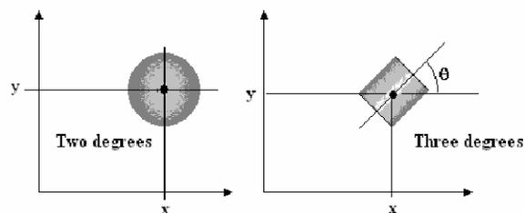
In order to completely specify the position and orientation of a cylinder in Cartesian space, we would need three coordinates x, y and z and three angles relative to each angle. This makes six degrees of freedom. A rigid body in space has  $(x, y, z, \theta_x, \theta_y, \theta_z)$ .
