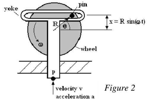
The pin is located at radius  $R$  from the centre of the wheel. The vertical displacement of the pin from the horizontal centre line at any time is  $x$ . This is also the displacement of point  $P$ . The yoke reaches a maximum displacement equal to  $R$  when the pin is at the top and  $-R$  when the pin is at the bottom.
