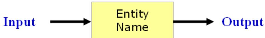
**Architecture.** All entities that can be simulated have an architecture description. The architecture describes the behavior of the entity. A single entity can have multiple architectures. One architecture might be behavioral while another might be a structural description of the design.
